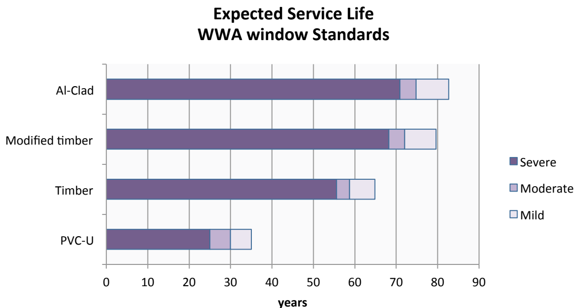
Figure 2.3 Expected Service Life for WWA window standards (Factors A, B, C, E and G)
